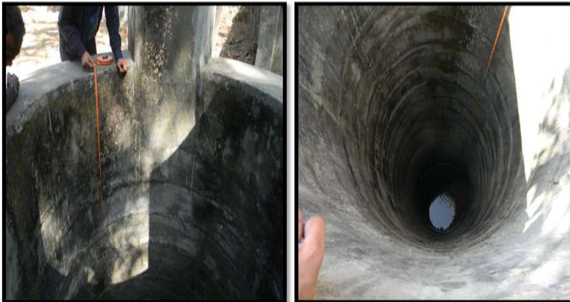
Figure-3: Measuring groundwater level depth at well.
