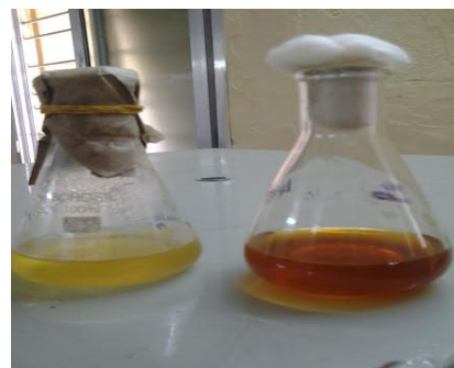
Figure 2. Picture of flasks A and B containing Aspergillus sps. culture filtrate before and after exposure to \text{Ag}^+ ions 24 hours.
