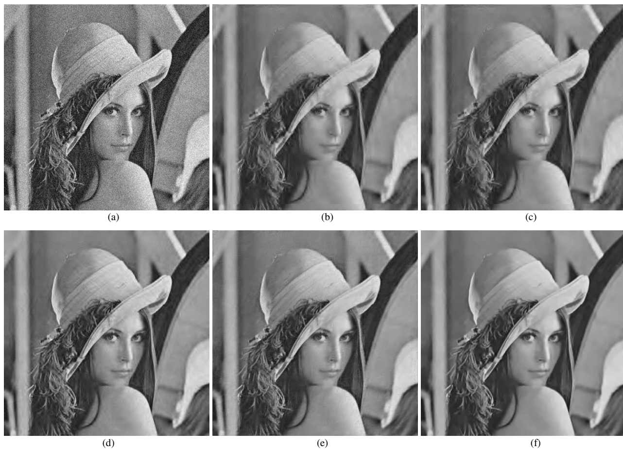
Fig. 2. Denoising of Lena image using various wavelet based methods. (a) Image with noise variance 20. (b) Soft thresholding (c) Cycle-spinning (d) Neighshrinksure (e) Multispinning (f) Proposed method.
