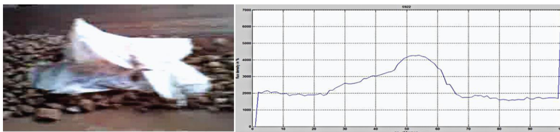
Figure2. A non-magnetic object on moving conveyor and its equivalent increase in white pixel count
