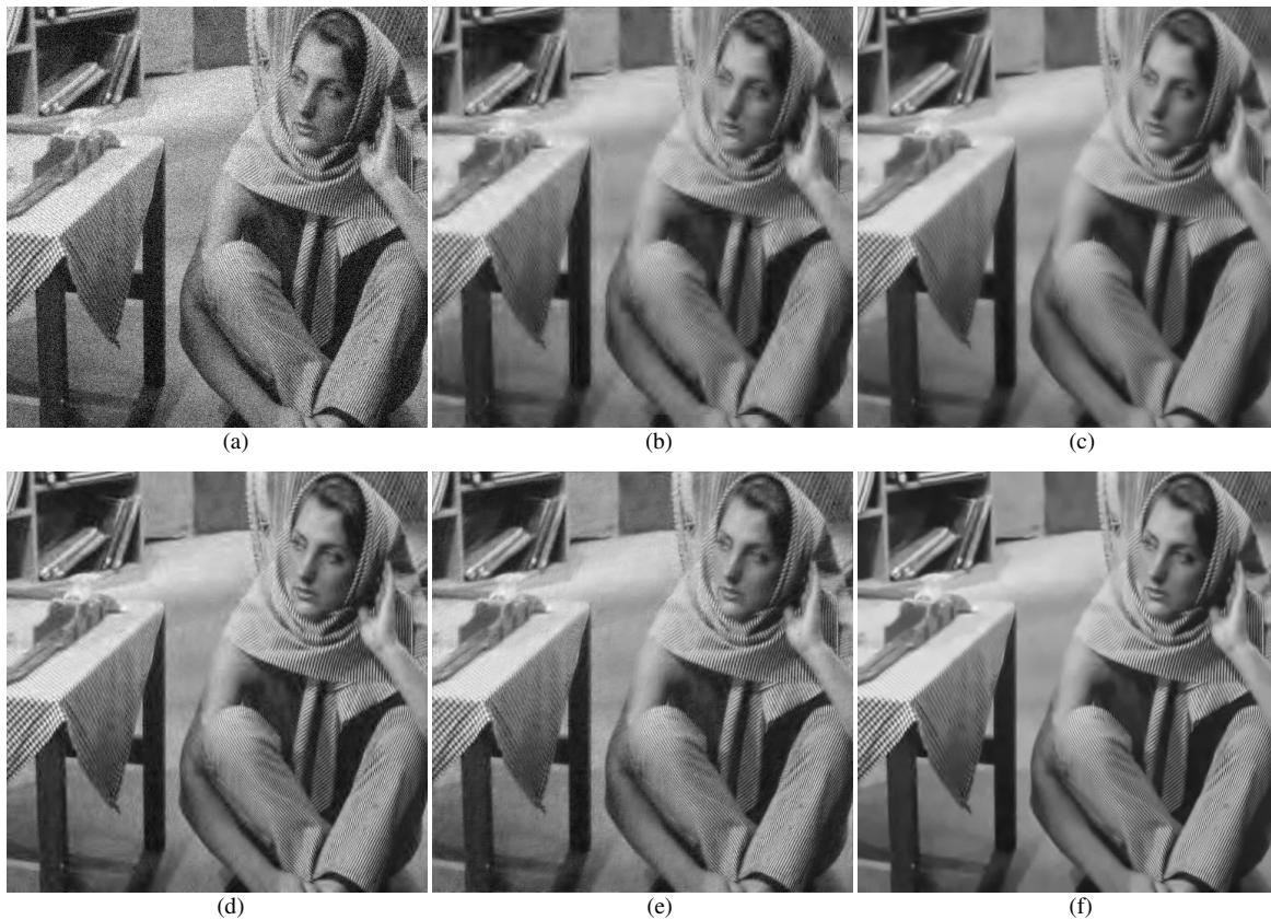
Fig. 4. Denoising of Barbara image using various wavelet based methods. (a) Noisy image with noise variance 20. Denoised by (b) Soft thresholding (c) Cycle-spinning (d) Neighshrinksure (e) Multispinning (f) Proposed method.
